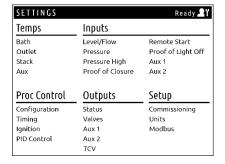
A valid password must be entered when prompted in order to adjust any setting. Each setting has a pre-determined security level based on its potential safety and reliability impact, and each security level has a separate password.
