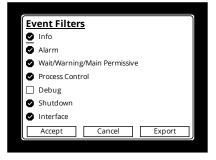
Use the event log filter to view specific events on the system screen. All event types will still be logged to the USB storage device, regardless of the filters selected.
