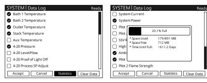
Use the Data Log Statistics window to see an estimate of how long the system will run before the USB storage device becomes full. Once full, the oldest data will be deleted and replaced with new data.
