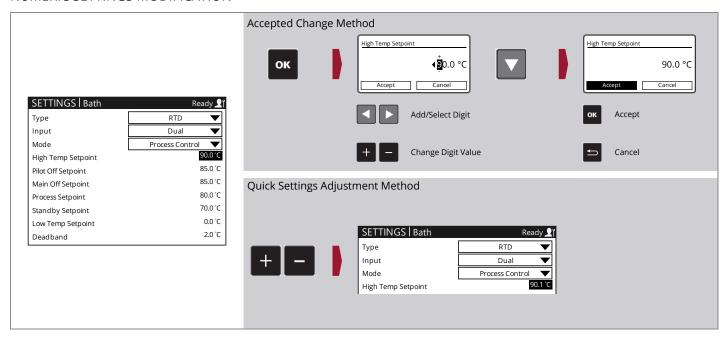
Settings changes made using the Quick Settings Adjustment methods take effect immediately when changed. Settings changes made using the Accepted Change method do not take effect until after the change has been accepted by the user. When using the accepted change method, pressing will discard a change that has not yet been accepted by the user.
