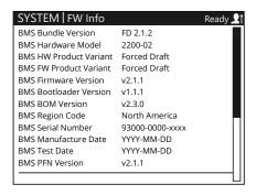
Refer to the controller's Information Screen (System > Firmware > Info) to find the hardware and firmware versions of your system.
